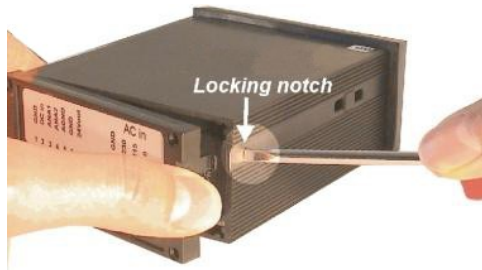
Removal of the back panel
